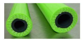
This moves away from the traditional coolant hose construction, all of our POSH range combines added security by providing a minimum of <u>4 plies</u>, combined with a <u>2mm</u> tube liner and the woven fabric (Meta-Aramid) also reduces the amount of dilation in the hose and hence, reduces the tendency for flex cracking.
